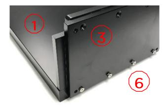
The baseplate  $\bigcirc$  is connected with the side panel  $\bigcirc$  by using countersunk screw M6 x 35  $\bigcirc$
